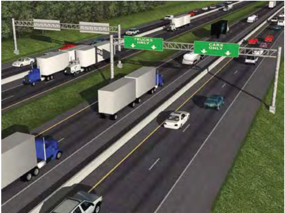
STAR Solutions, a group of investors, is proposing widening I-81 from 4 to 8 lanes with trucks operating separately as shown in this visualization. From STAR Solutions, Richmond, Virginia.
