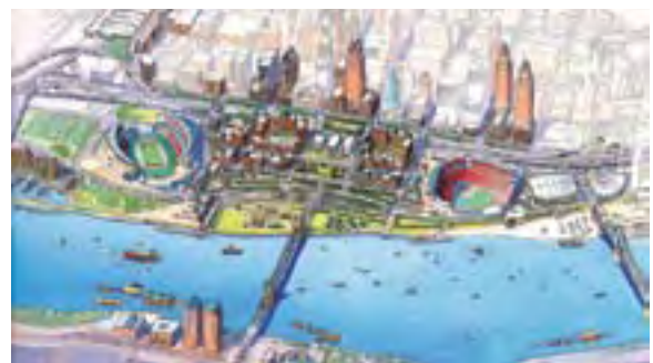
Plan for eventual lidding of Fort Washington Way. It was rebuilt in 1996-2000 to allow this by eliminating multiple downtown ramps.
