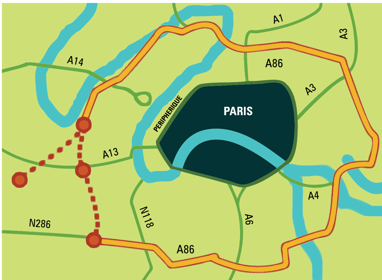
The A86 tunnelways will complete a missing link in the A86 outer beltway around Paris. The low-vehicles doubledeck tunnel now under construction is 6 miles long, and the 4.7 mile long all-vehicles tunnel heading off to the west is to be built later. Map from Cofiroute.
