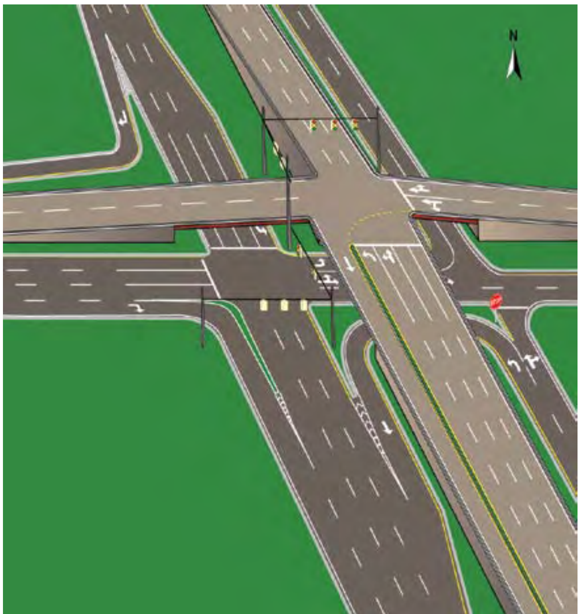
The Echelon Interchange by Miller Consulting is very similar to the HICIS.
