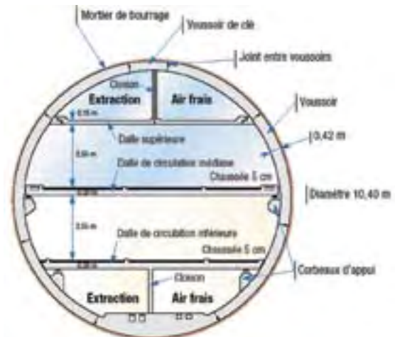
Dimensions of the A86 West tunnelway project. Within a 34-foot (10.4m) diameter tube built with a tunnel-boring machine, two decks provide 8 feet 4 inches overhead clearance for three levels plus a pair of ten foot travel lanes plus a breakdown shoulder lane. Drawing from Cofiroute.
